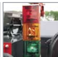
Overload warning lamps + auto stop + alarm
